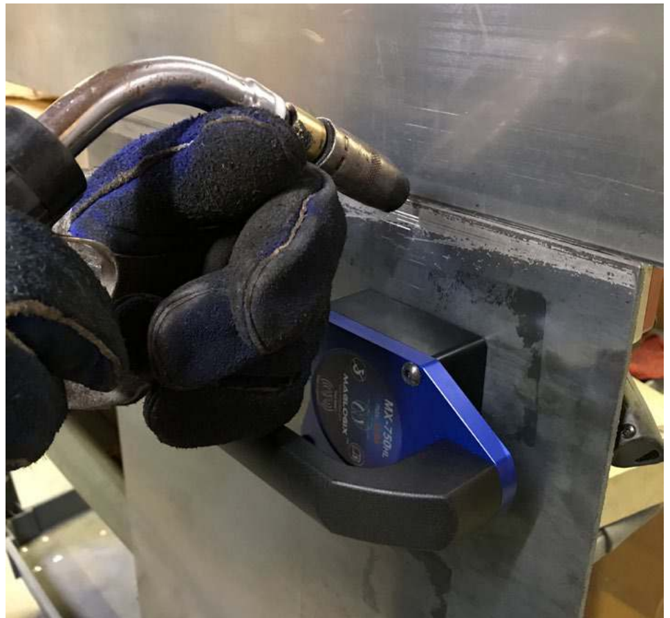
Pictured is a Maglogix HandLifter. These magnets can replace tack welds, enabling maintainers to weld very close without affecting the welding arc. These magnets can also be used as a hand rest, which reduces operator fatigue and increases safety. (Photo by Ted Brooks, courtesy of Maglogix.)
