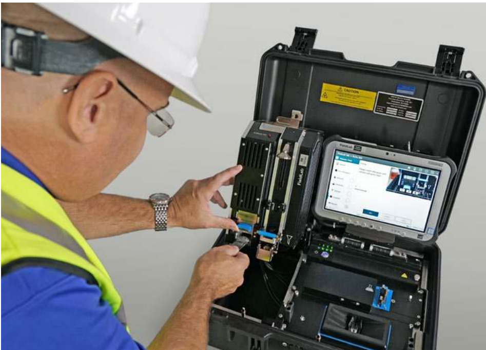
The Spectro FieldLab 58 is a portable fluid testing and diagnostic tool that indicates fluid chemistry contamination, viscosity, and other measures of health. (Photo courtesy of AMETEK/Spectro Scientific.)
